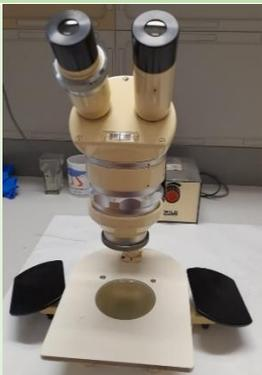
A photograph of a WILD stereomicroscope. It is a light-colored, binocular microscope with two eyepieces on top and a large objective lens at the bottom. The brand name 'WILD' is visible on the front.                                |
