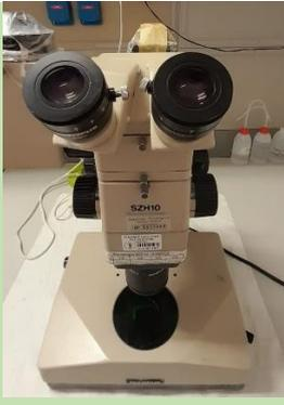
A photograph of an Olympus SZH10 stereomicroscope. It is a light-colored, binocular microscope with two eyepieces on top and a large objective lens at the bottom. The brand name 'OLYMPUS' and model 'SZH10' are visible on the front. |
